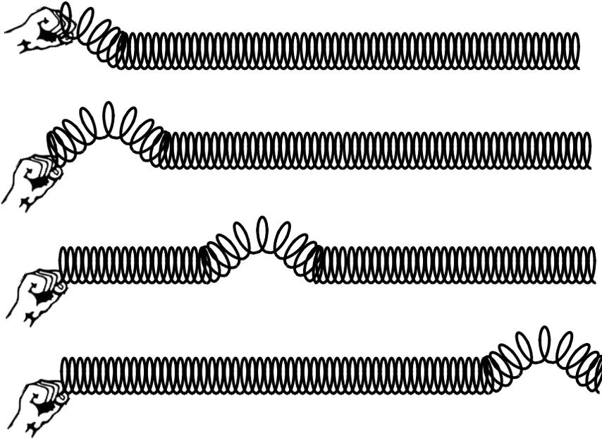
Most students will notice that they can send waves where the hump is a different height (amplitude). Use a meter stick to measure the heights.
