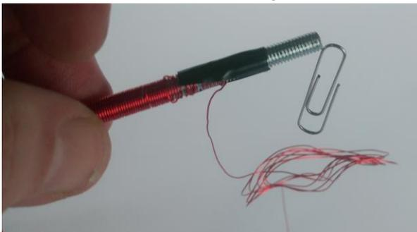
Note: The magnet wire can get very hot, so only connect it to the battery for a few seconds at a time.
