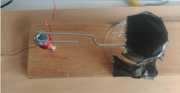
7. Insert the D-cells into the battery holder. Connect one alligator clip between one battery terminal and one of the ends of the magnet wire.
